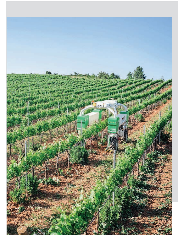
TED adapts to vineyards thanks to two arch heights (2.00 m or 2.35 m). It features the widest arch on the market (1.05 m).
