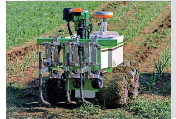
RTK GPS ensures centimeter accuracy. The work maps produced during sowing or furrow tracing are used for the entire technical itinerary.
