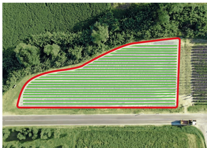
The geofencing prevents the robot from leaving the work area.
