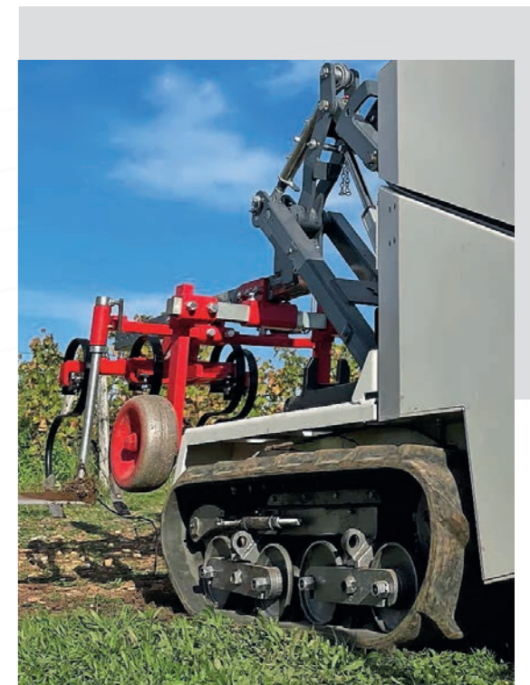
The Boisselet saddle can hold a standard pole or a 3-point lift.
